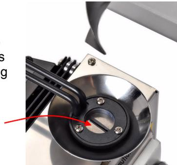
The helical mixing blade creates excellent laminar and chaotic flow within the melt chamber, allowing the entire melt to experience a uniform processing history.
