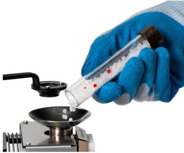
2. Melt the materials in the chamber, and then mix them with the hand tool, or an overhead mixer positioned over the Model-M device.
