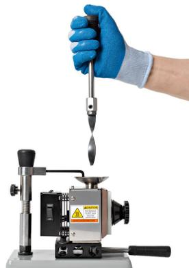
Move the melt chamber to the Model-S machine and make an injection molded part with the mixed material.
