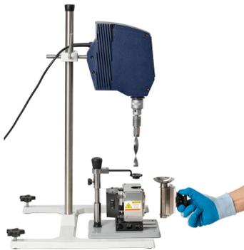
4. Insert the melt chamber into the Model-S Injection Molder.
