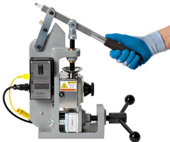
6. Remove the mold from the Model-S machine, and then remove the injection molded part from the mold.
