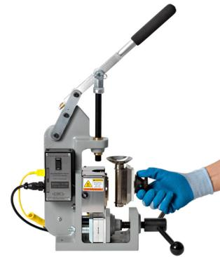
5. Inject the mixed material into a desired mold by pulling down the handle of the model-S machine.
